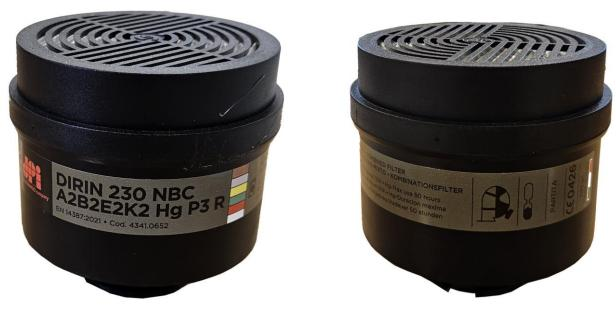
Special combined filter Dirin 230 NBC A2B2E2K2HgP3 type A2B2E2K2HgP3 connected to full face mask provides protection of respiratory system of user against organic gases and vapours with a boiling point above 65°C, inorganic gases and vapours (excluding carbon and nitrogen monoxides), sulphur dioxide and other acid gases, ammonia and organic ammonia derivates, mercury vapours, solid and liquid aerosols in accordance with the information supplied by the manufacturer.
